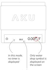
Live flow rate display can be turned On/Off in setting mode (see page 11)
